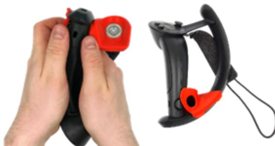
Push on the two sides of the MagCup to slide it on the round part of the controller. Make sure to push out the sides enough, otherwise you may scratch your controllers.
