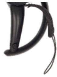
Put back the string of the controller's hand strap by pushing the spring button.
