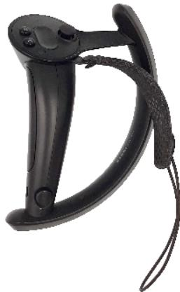
Put back the string of the controller's hand strap by pushing the spring button.
