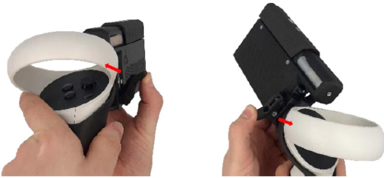
Clip the first clamp. Use the provided Allen key to loosen the screw and adjust the tightness.
