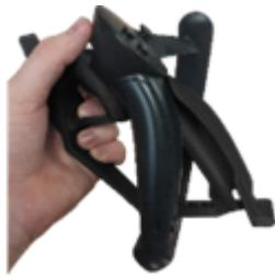
Detach the strap's string from the controller and put the cup into the controller's handle, like shown in the picture above.
